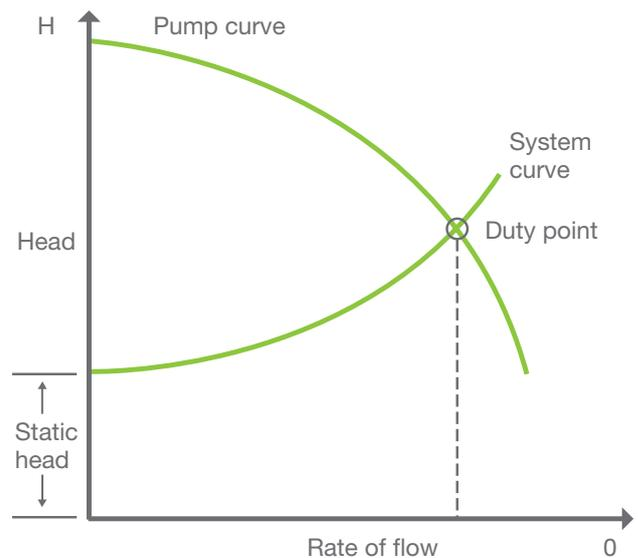
**Figure 12: The duty point of a pump.<sup>3</sup>**
