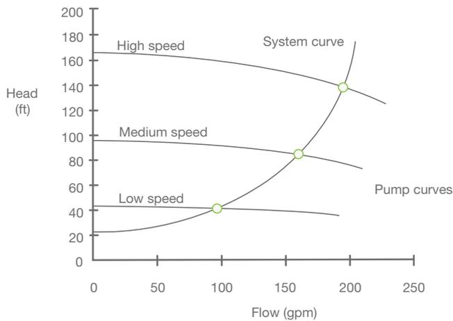
**Figure 6: Multiple-speed pump characteristic curves.**<sup>9</sup>
