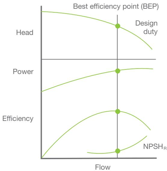
**Figure 11: A simplified centrifugal pump characteristic curve.<sup>9</sup>**
