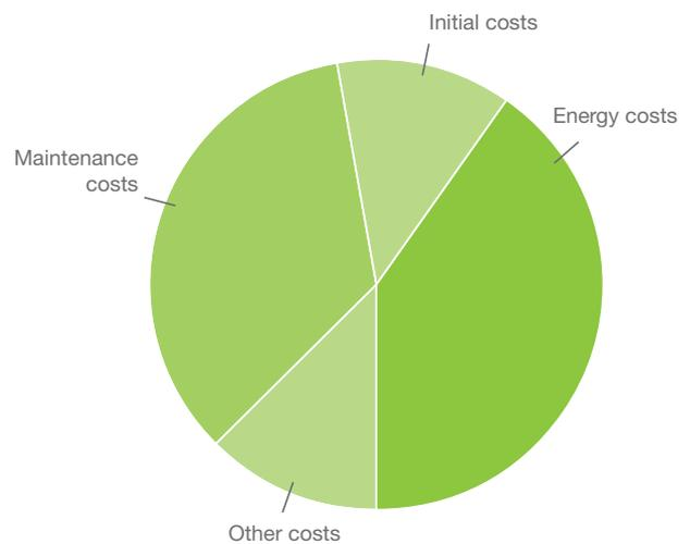
Figure 1: Typical proportions in the life cycle cost analysis for a medium-sized industrial pump.<sup>3</sup>
