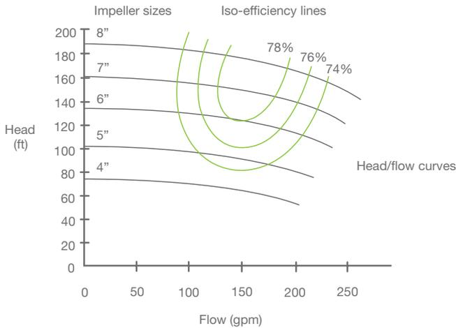
Figure 5: Performance curves for different impeller sizes.<sup>9</sup>
