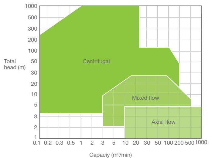
**Figure 10: Centrifugal pump types and ranges.<sup>14</sup>**
