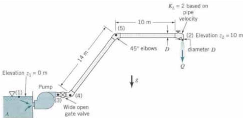
Figure 9: A simple pumping configuration diagram.<sup>13</sup>
