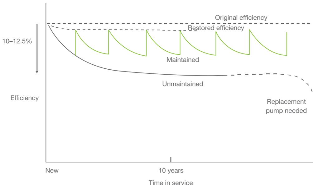
Figure 8: Average wear trends for maintained and unmaintained pumps.<sup>2</sup>
