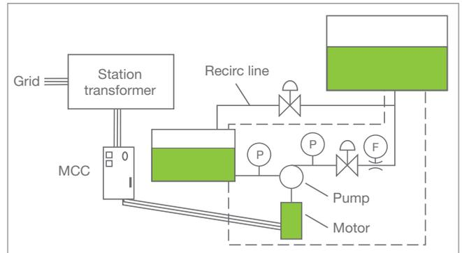
**Figure 3: Calculating pumping system efficiency.**<sup>6</sup>
