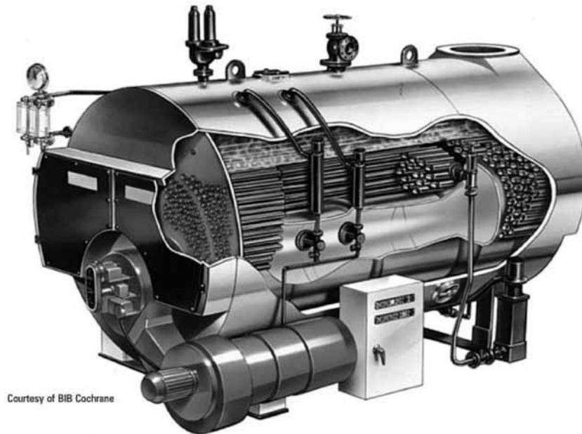
Figure 6: Modern package boiler.<sup>8</sup>
