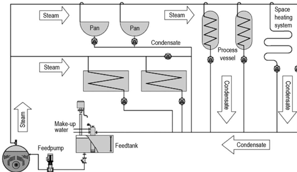
**Figure 4: Typical basic steam circuit.<sup>8</sup>**
