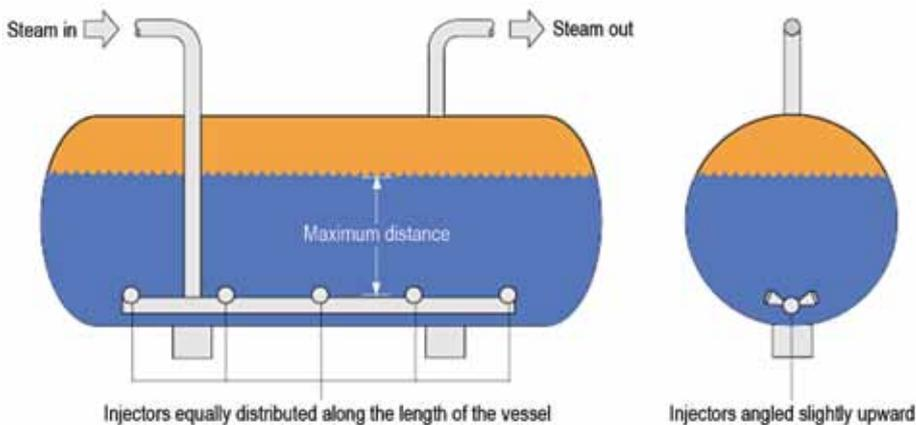
Figure 13: Steam accumulator (side and end view).<sup>8</sup>
