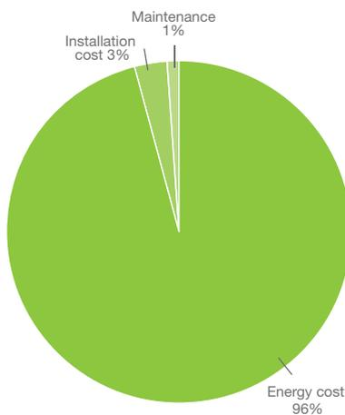
Figure 1: Typical lifecycle costs of a steam system.<sup>1</sup>
