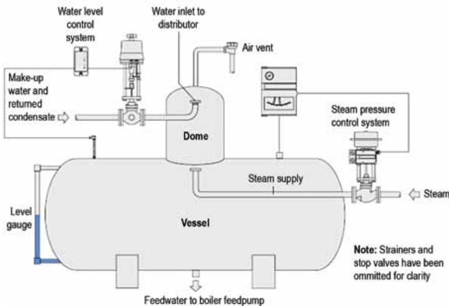
Figure 8: Pressurised de-aerator.<sup>8</sup>
