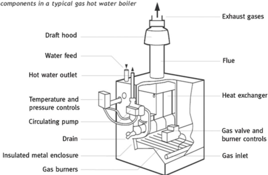
Figure 14: Typical gas-fired hot water system.<sup>10</sup>
