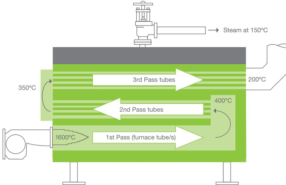
Figure 5: Typical flow path through fire-tube shell boiler.<sup>8</sup>
