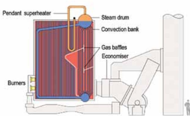
Figure 7: Water tube boiler.<sup>8</sup>
