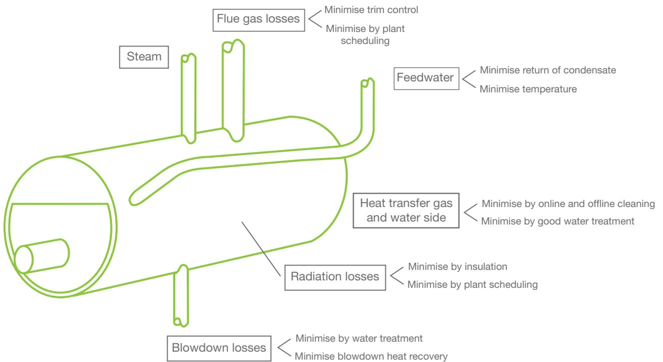
Figure 2: Typical boiler losses for a shell boiler.<sup>4</sup>
