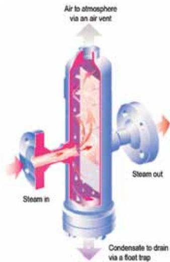
Figure 11: Cut away section of a separator showing operation.<sup>8</sup>
