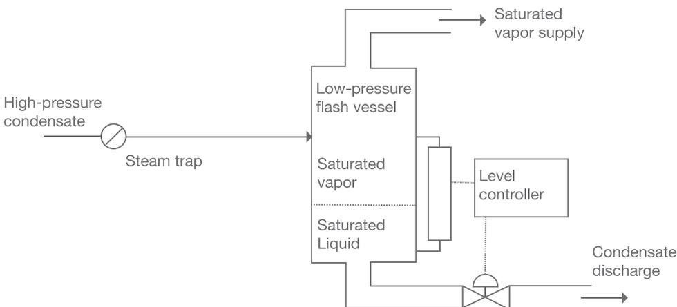
Figure 3: Flash steam recovery vessel.<sup>5</sup>
