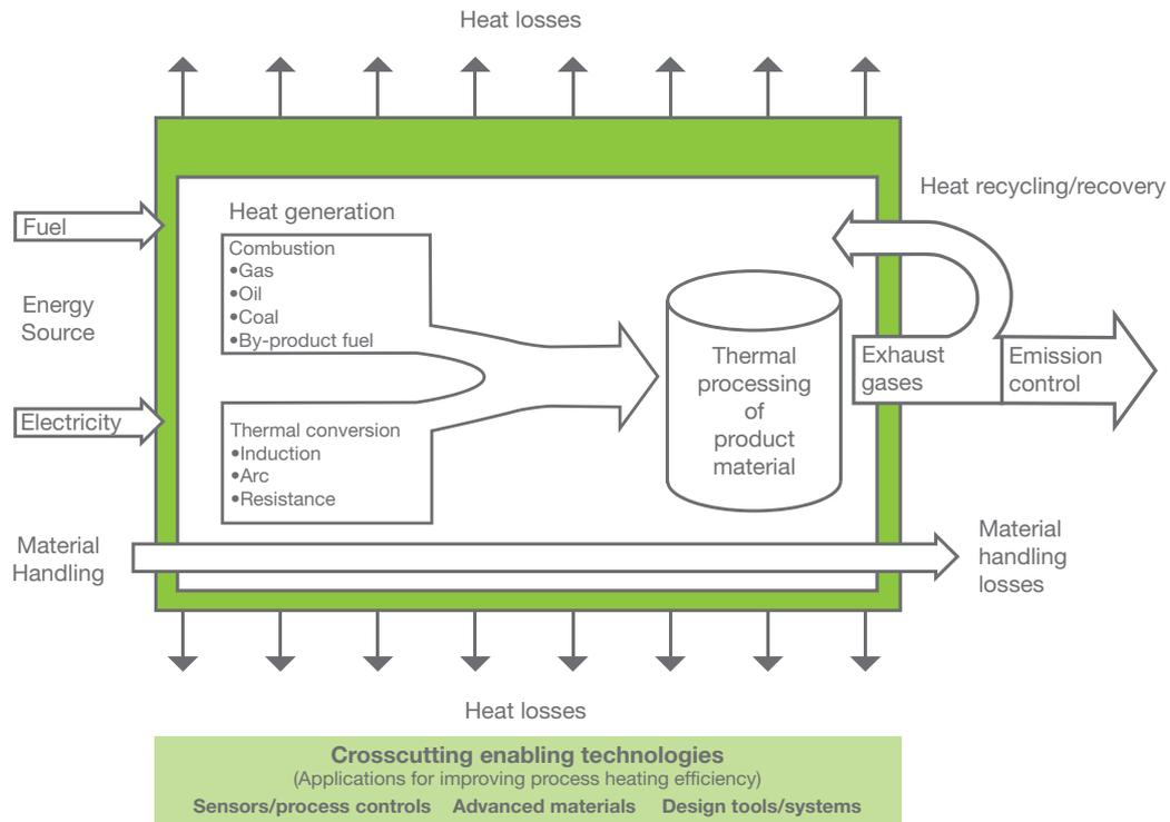
**Figure 15: Key components of a process heating system.<sup>2</sup>**
