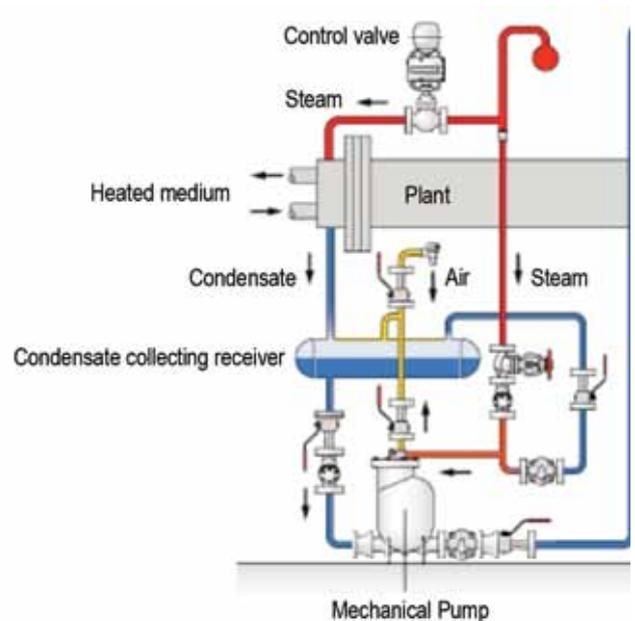
Figure 12: Condensate return system.<sup>8</sup>
