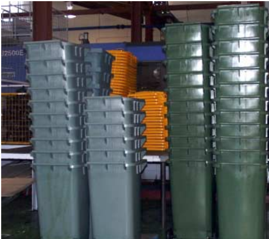
Figure 5: A collection of garbage bins made from modified milk bottle HDPE
