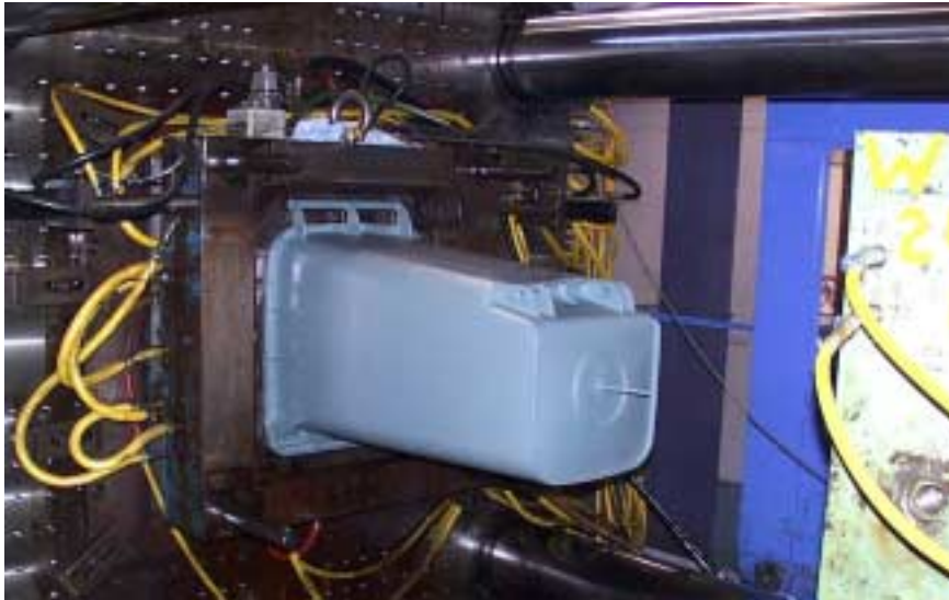
Figure 4: A mobile garbage bin in the injection moulding machine prior to removal, made entirely from reactively modified recycled milk bottle HDPE
