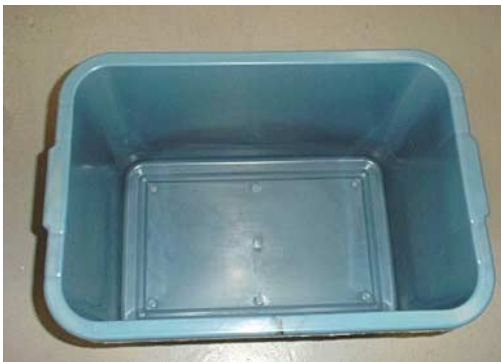
Figure 3: A crate moulded entirely from reactively modified recycled milk bottle HDPE
