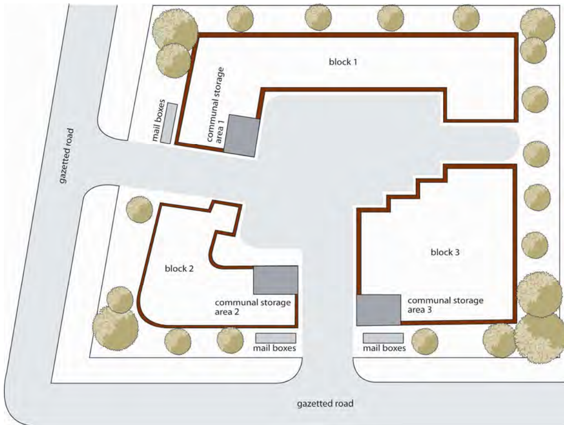
Figure 4-2 Example of Option 2: bulk bins used for garbage and MGBs for recycling
