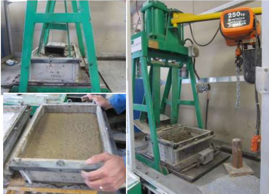
Figure 15. Slab compaction using BP compactor at an external laboratory facility
