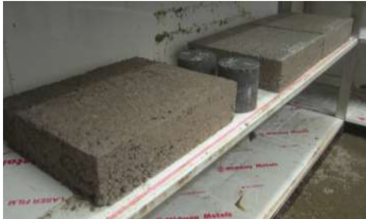
Figure 16. Compacted slabs in fog room
