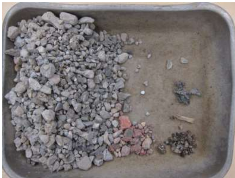
Figure 1. Foreign material contents in crushed concrete
