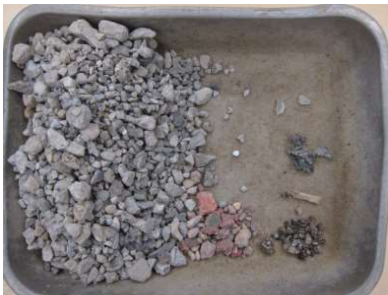
Figure 1. Foreign material contents in crushed concrete
