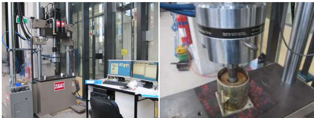
Figure 4. CBR test using MTS-250kN
