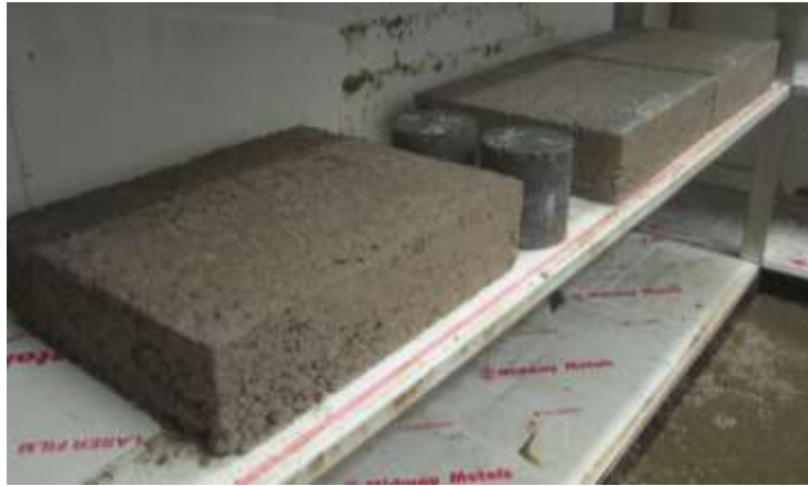
Figure 16. Compacted slabs in fog room
